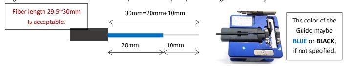
0.250mm Primary Coating: 20mm, and 0.125mm Bare Fiber: 10 mm
